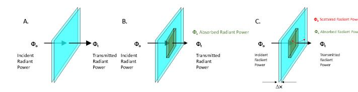
Figure 1: Diagrammatic representation of theoretical attenuation by a thin layers of non-attenuating (panel A), absorbing (panel B), and absorbing and scattering (panel C) material. The thickness of the layer is given by  $\Delta x$ .
