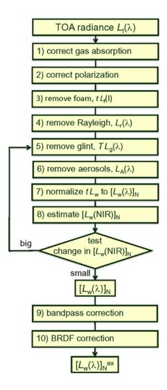
Figure 1: Flowchart of the atmospheric correction process.
